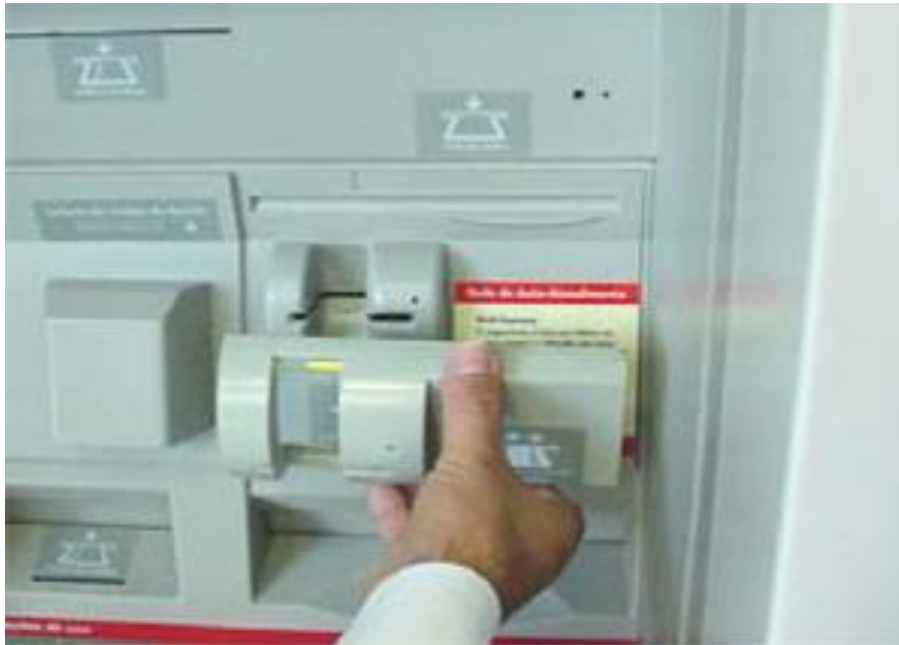
Photo 1: False slot fixed to the original card slot (same colour and sticker). Contains additional card reader to copy information and duplicate your card.
