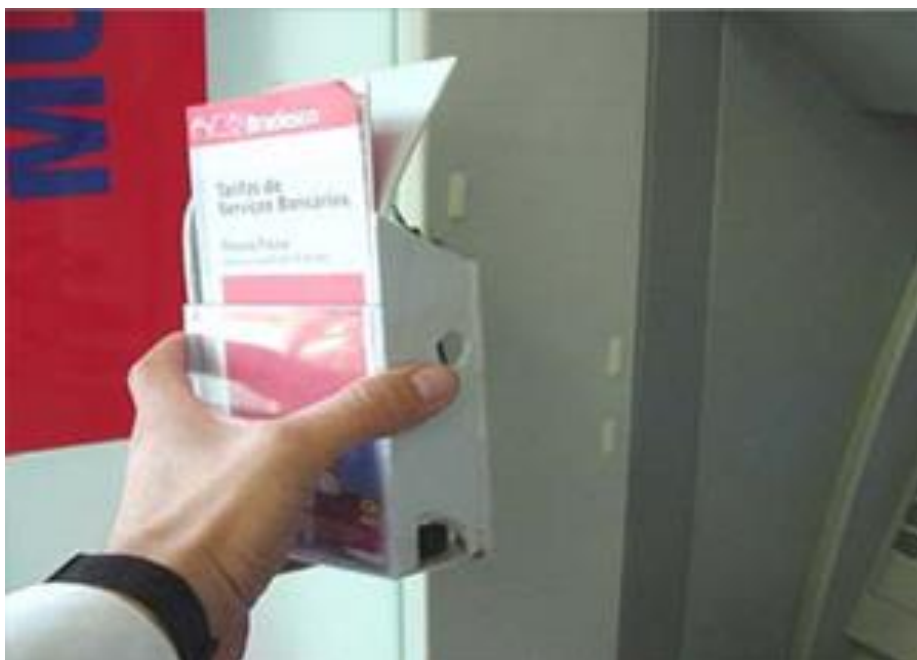
Photo 2: The side of the box facing the ATM screen has a reflective glassy hole. That's a camera!
